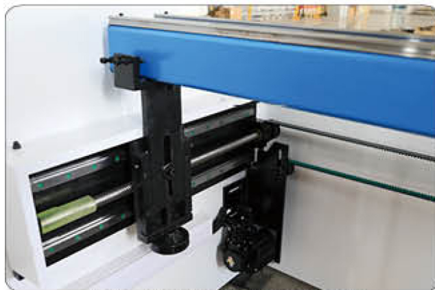
Increase the double linear guide rail after the stopper, ball screw linear guide rail
