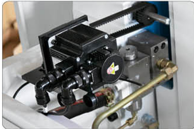
The servo motor drives the cylinder
