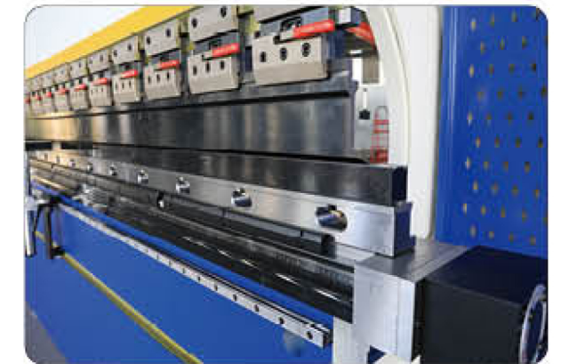
Mechanical compensation, numerical control tooling(punch & die)
