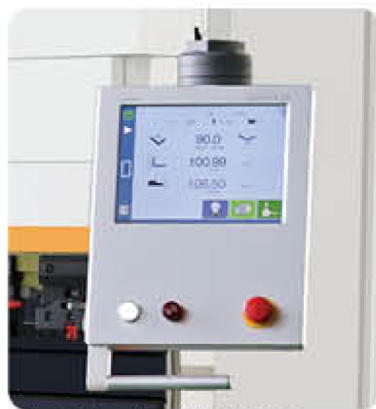
The Switzerland CYBELEC Company CYB T12 Numerical control system of bending machine
